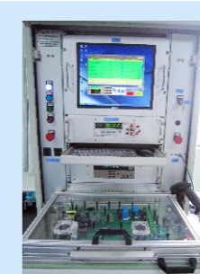
Automatic PCBA ATE test platform
